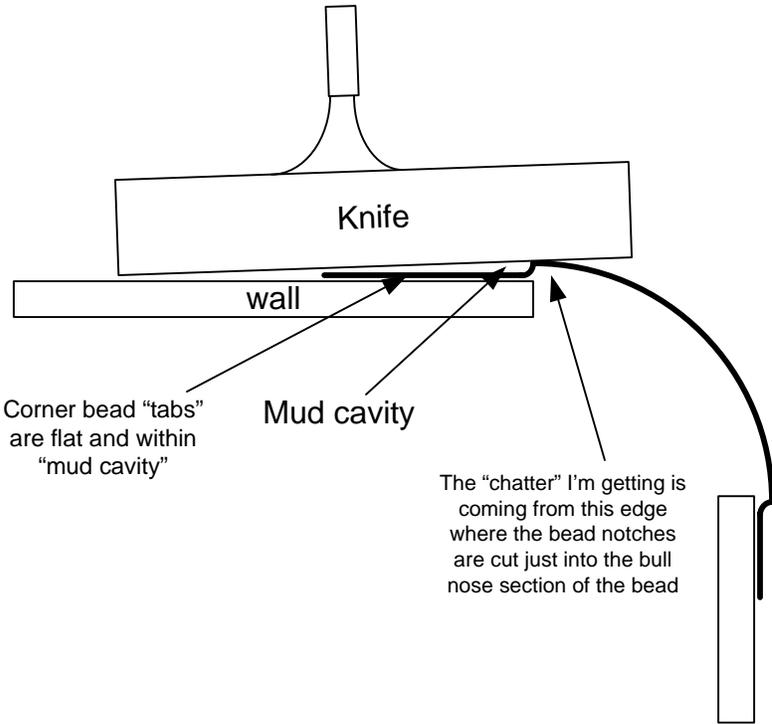
Notches of the arch bead extend just out of the "mud cavity" and into the "bullnose" part of the bead.
